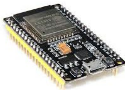
Gambar 1. Board Mikro Controller ESP32
